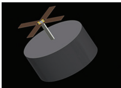
▲ Fig. 2 Deployed antenna elements on a cylindrical satellite.
